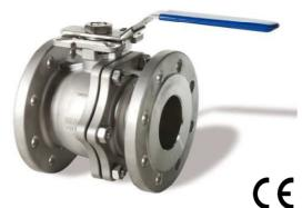
Shut-off ball valve split-body type with the body in stainless steel CF8-M with a floating ball, manufactured in accordance with the most severe product standards and the quality management of ISO 9001.
